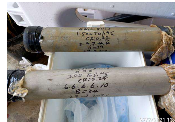
Collecting Soil Samples at 0.5m bgl
