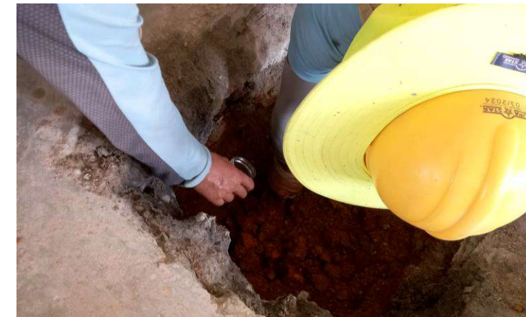
Collecting Soil Samples at 0.5m bgl
