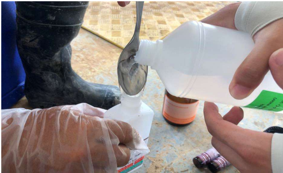
Collecting Equipment Blank for Soil Sampling
