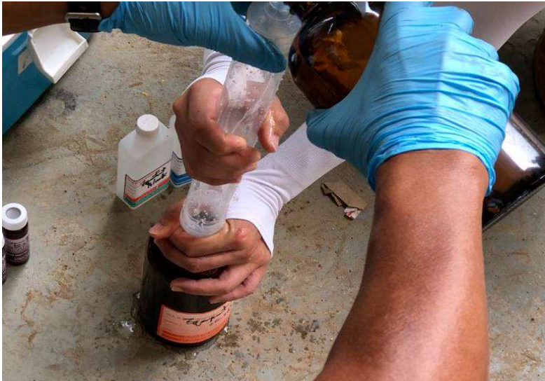
Collecting Equipment Blank for GW Sampling
