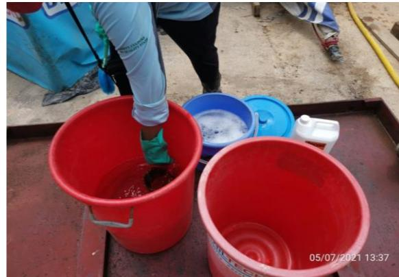
Cleaning with lab-grade detergent and distilled Water
