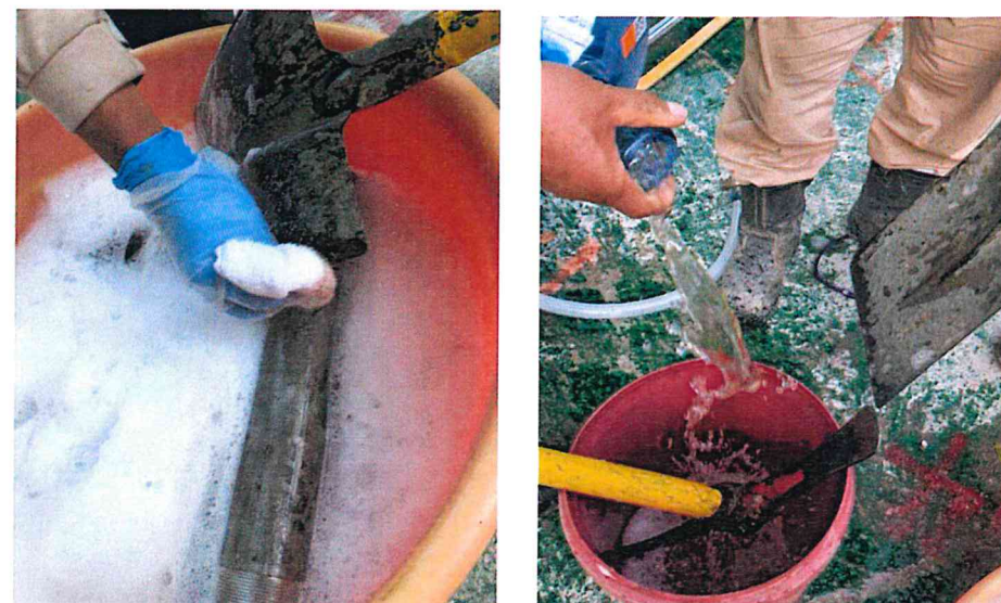
Cleaning with lab-grade detergent and distilled Water
