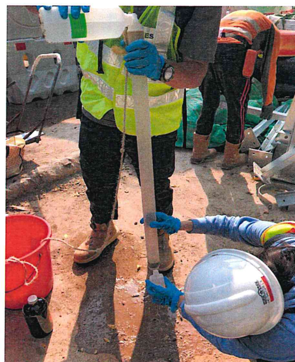
Collecting Equipment Blank for GW Sampling
